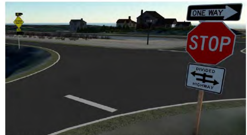
Figure 6. Second view of divided highway intersection show animated flashing beacons on warning sign.
