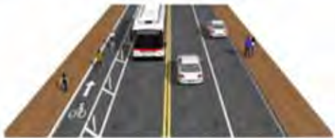
Protected Contraflow Lane
