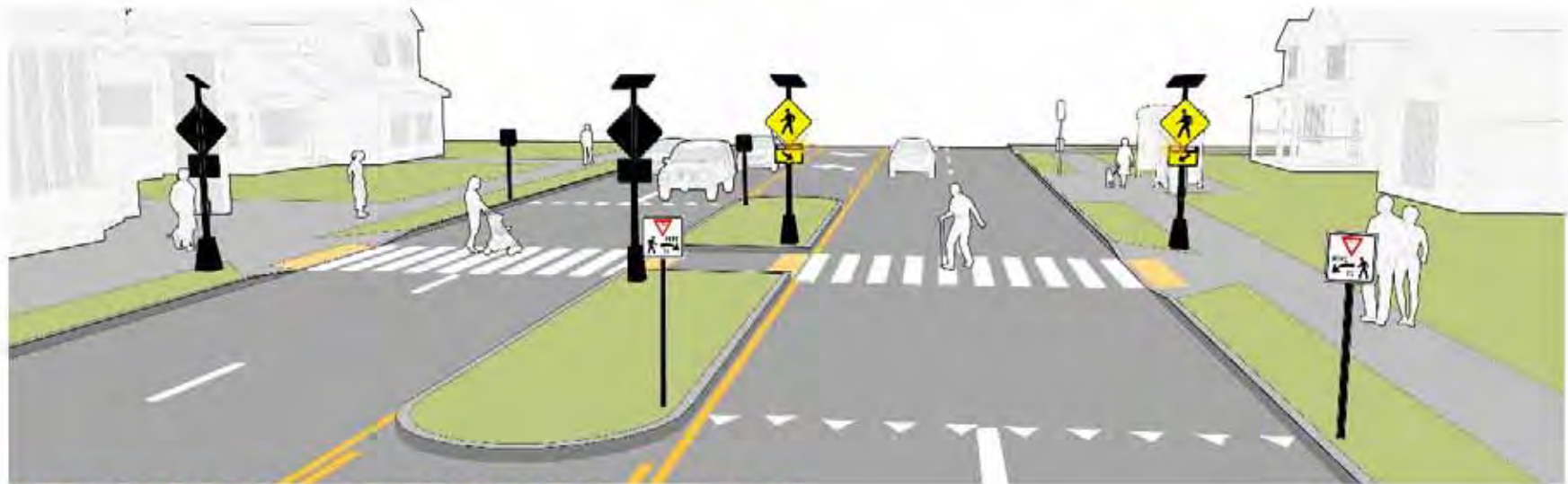
RECTANGULAR RAPID FLASHING BEACON AND CROSSING ISLAND
