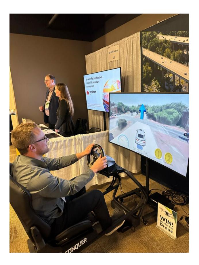
This driving simulator takes reality capture data (such as LiDAR, point clouds, or photogrammetry) and creates interactive visualizations. The simulations aren't just limited to steering wheel controls, they can be JMT Technology Group's virtual spaces platform to help create interactive experiences, simulations, and virtual tours that stakeholders can access via the web with keyboard controls or their mobile devices.
