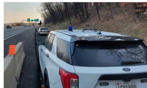
Temporary installation of blue light
