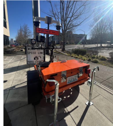
Example of an unmanned unit from Washington State DOT.
